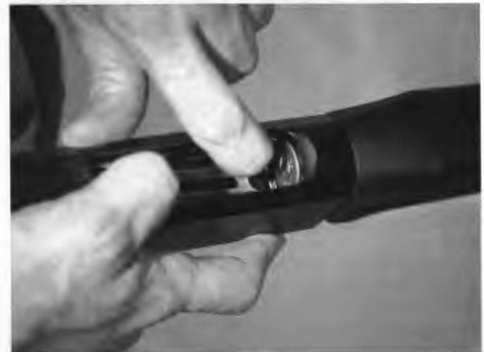
Close the action and turn the gun over. As the firing side thumb holds the carrier up, the support side index finger depresses the shell stop to release the shells from the magazine.
