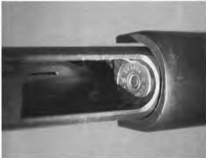
With the action open, the shell stop on the ejection port side is retaining the shell in the magazine.
