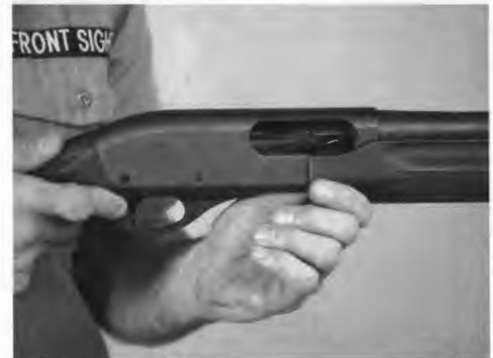
To unload the magazine on a Remington 870 leave the action open and push the carrier up out of the way.
