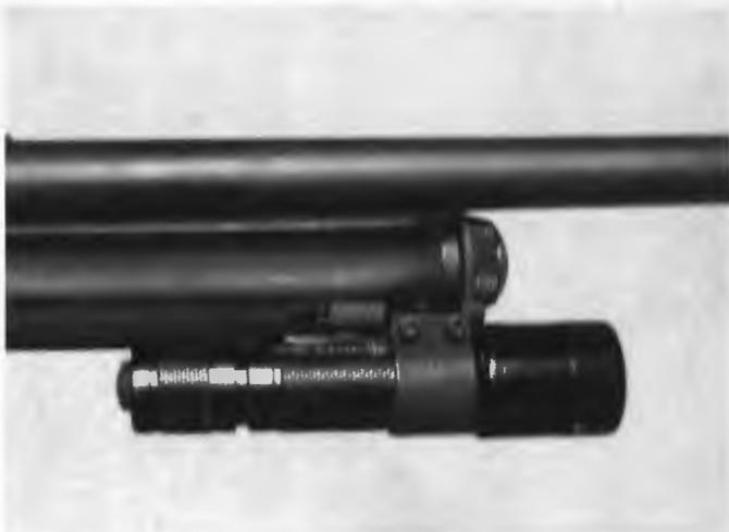
An inexpensive section of scope mounting rail can be used to mount a flashlight or weapon light.
