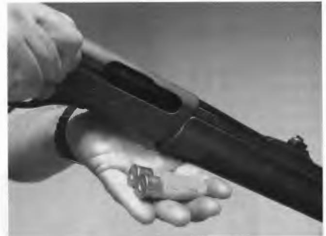
With Remington 1100 and 1187 semi-autos the next round can also be rolled off the carrier.
