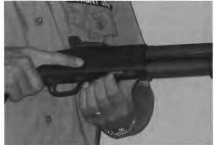
With Mossberg shotguns, the action must be closed to unload the magazine. The shell stop opposite the ejection port retains the shell.
