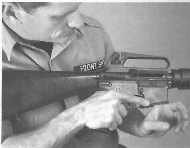
Insert the support hand index finger into the magazine well to ensure it is clear.
