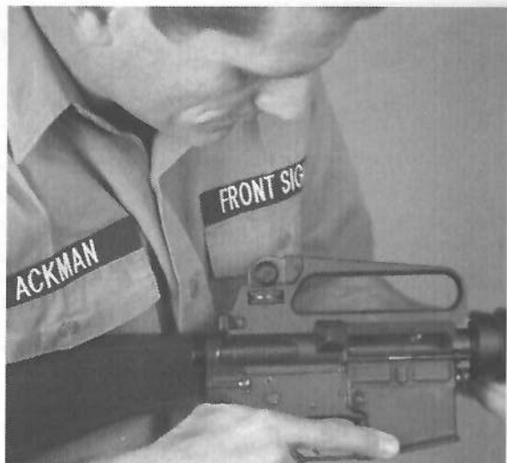
Once the bolt is locked to the rear, visually inspect the chamber.
