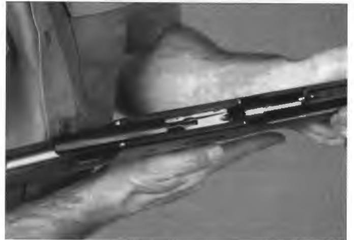
Once all rounds have been ejected, with the action open, look into the chamber to make sure it is clear. Close the action and check the magazine tube for rounds.
