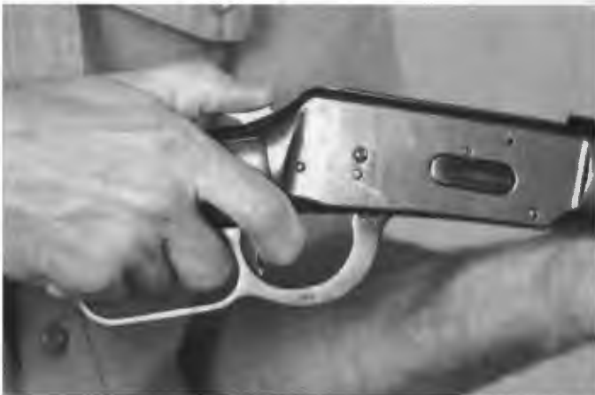
With the thumb on the hammer, press the trigger and ride the hammer forward to the half-cock position.
