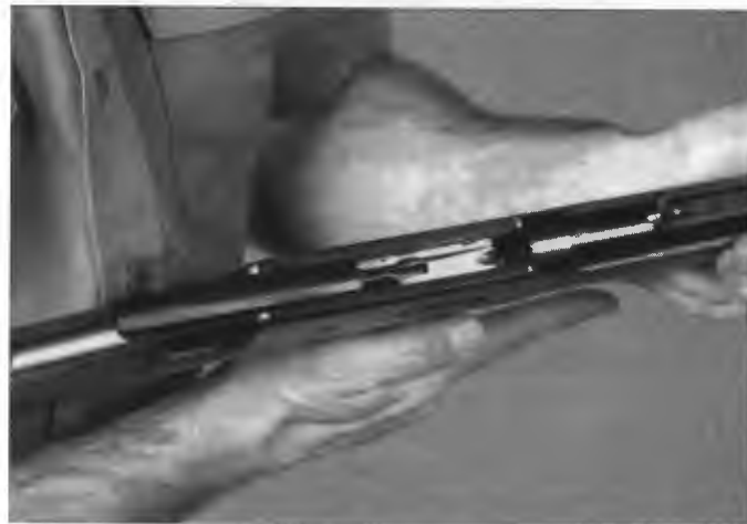
Once all rounds have been ejected, with the action open, look into the chamber to make sure it is clear. Close the action and check the magazine tube for rounds.
