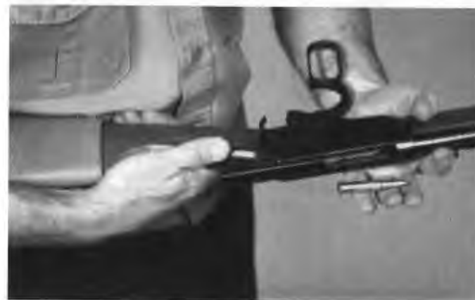
Support the weapon and use one hand to run the action to eject rounds into the other hand.
