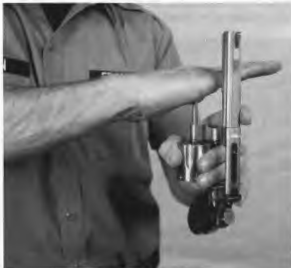
Trap the cylinder in the open position and rotate muzzle up. With the palm of the firing hand, strike the ejector rod to eject the cartridges from the chambers.
