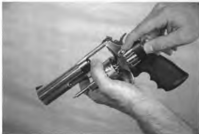
Properly index speed loader in firing hand.
