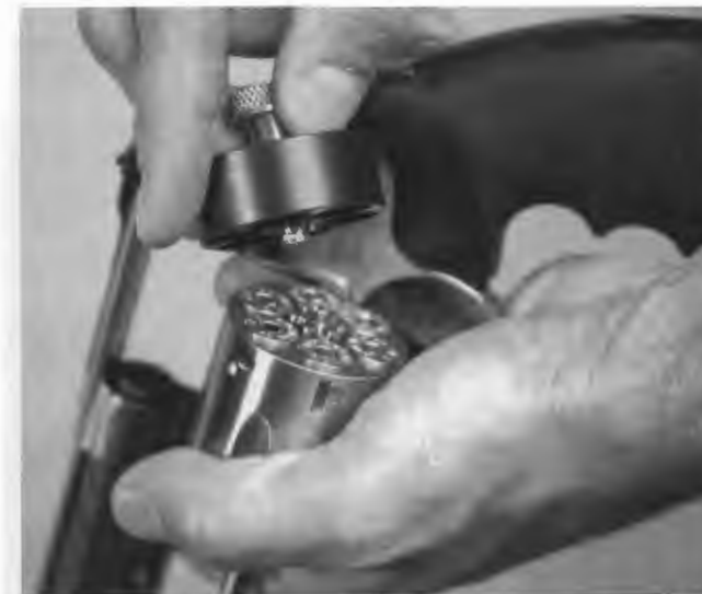
Align speed loader behind cylinder and insert rounds about half way into the chambers. Release the rounds into the chamber and drop the speed loader.
