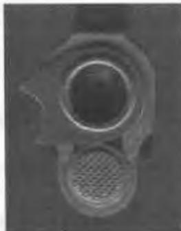
2. Remove plug. If plug does not come free easily, rotate plug in a counter-clockwise direction to separate plug from recoil spring
