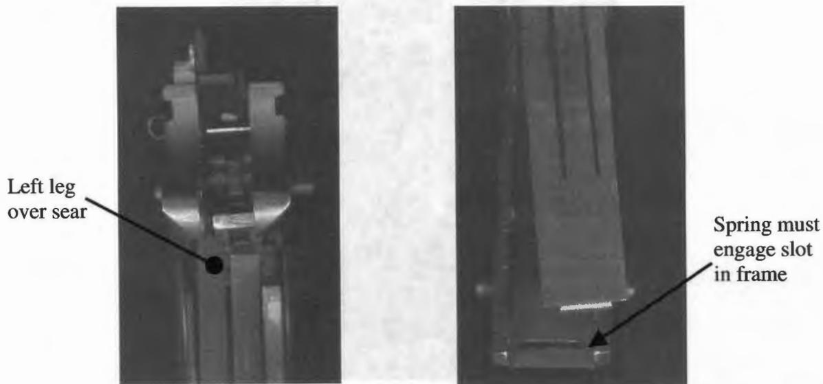
18. Slide the mainspring housing in place from the bottom of the frame, aligning the slots in the frame with the rails on the mainspring housing assembly until the mainspring housing is approximately 2/3 of the way up
