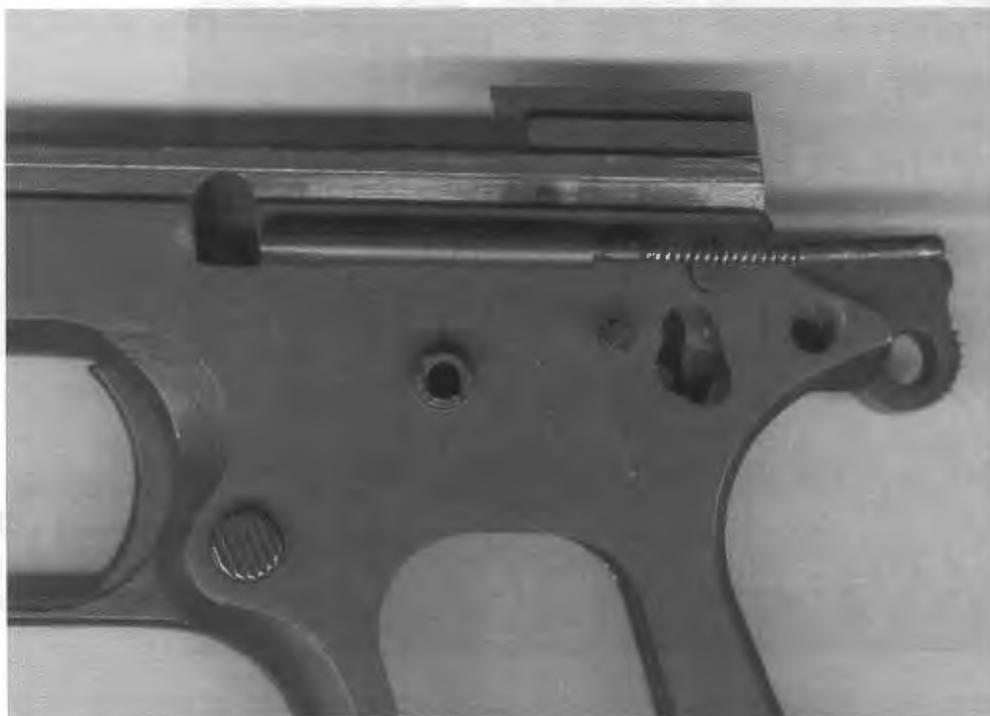
17. Raise the hammer strut and insert the sear spring into the rear of the frame
