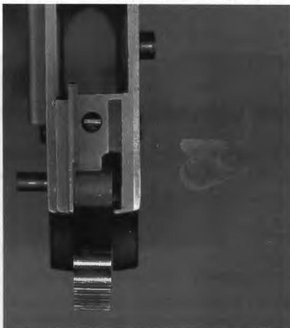
16. From the rear, insert the slide stop plunger, plunger spring and safety plunger into the plunger tube housing
