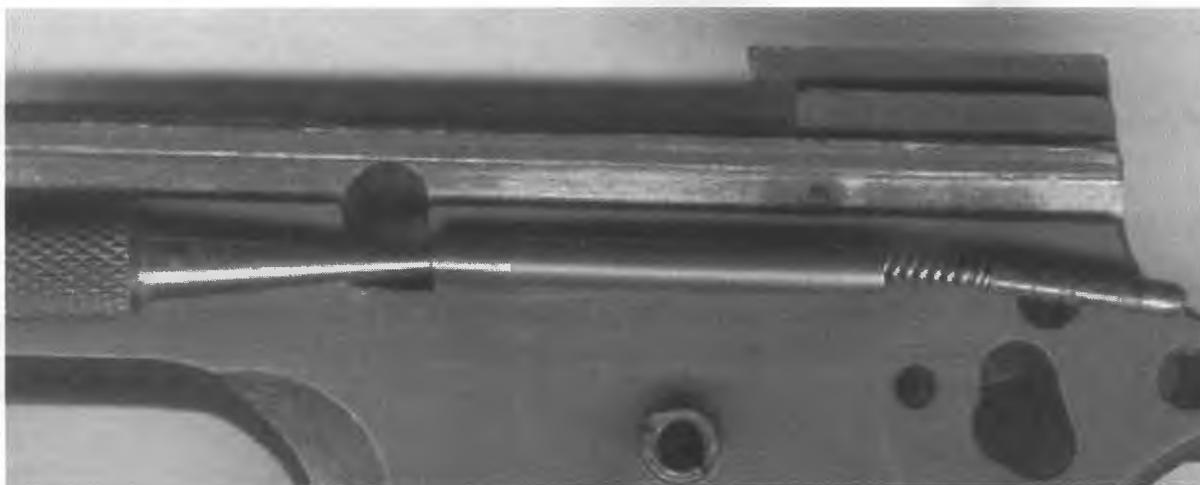
**Note:** Do NOT remove the ejector, plunger tube housing, or stock screw bushings
