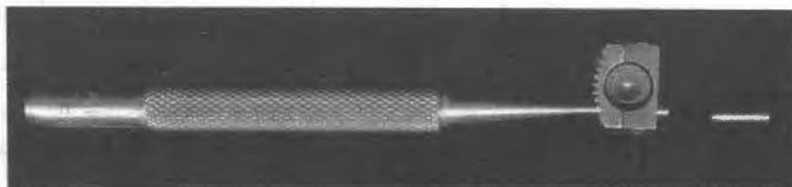
7. Remove the mainspring cap, mainspring, and mainspring housing pin retainer from the top of the mainspring housing
